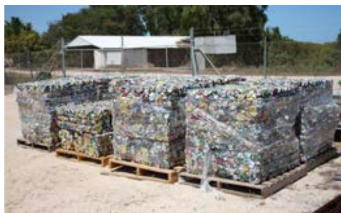
Best practices implemented in Pormpuraaw include crushing and baling aluminium cans prior to transfer, Pormpuraaw Aboriginal Shire, photo RAIN Pty Ltd.
